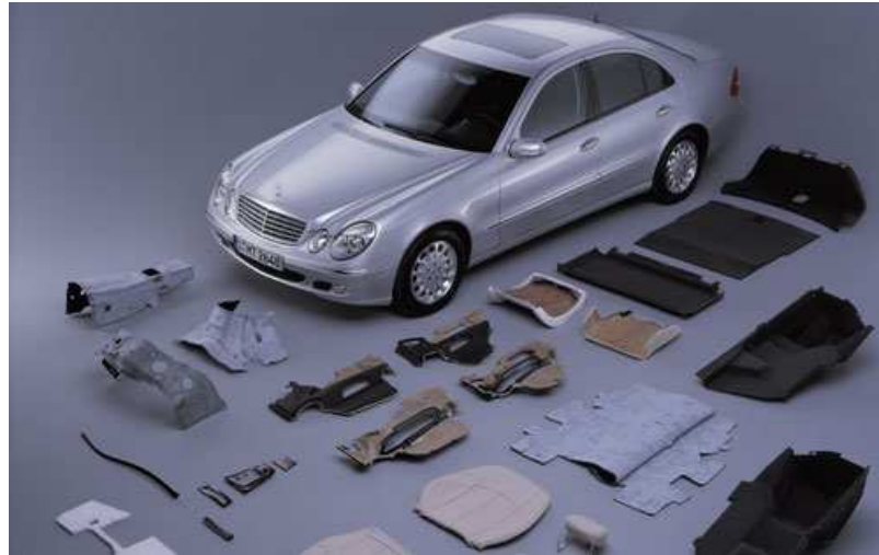
Figure 1: Automobile components made of natural fiber reinforced composites [13].
