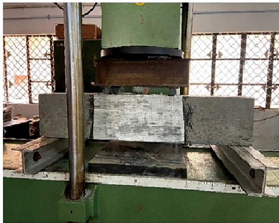
Figure 8: Test setup of glass fibre wrapped beams.
