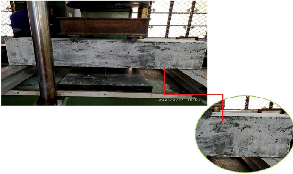
Figure 9: Failure of conventional shear deficient RC beams.
