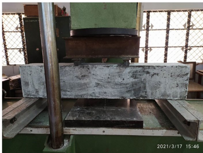
Figure 6: Test setup of conventional beam.
