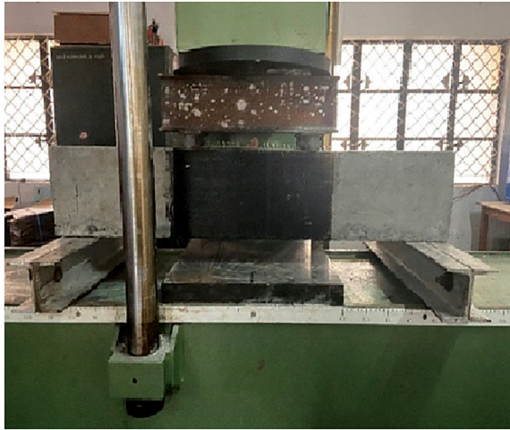
Figure 7: Test setup of basalt fibre wrapped beams.
