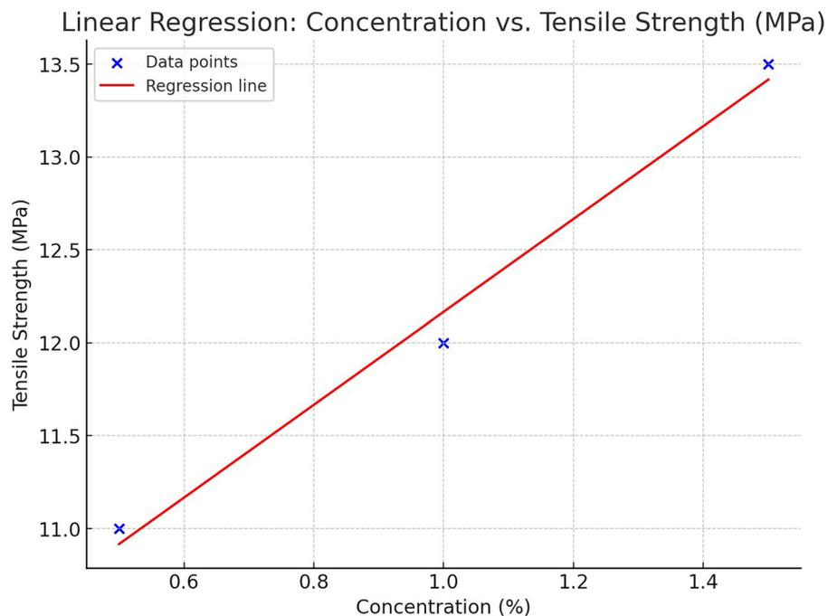
Figure 12: Linear Regression: Concentration vs. Tensile Strength.
