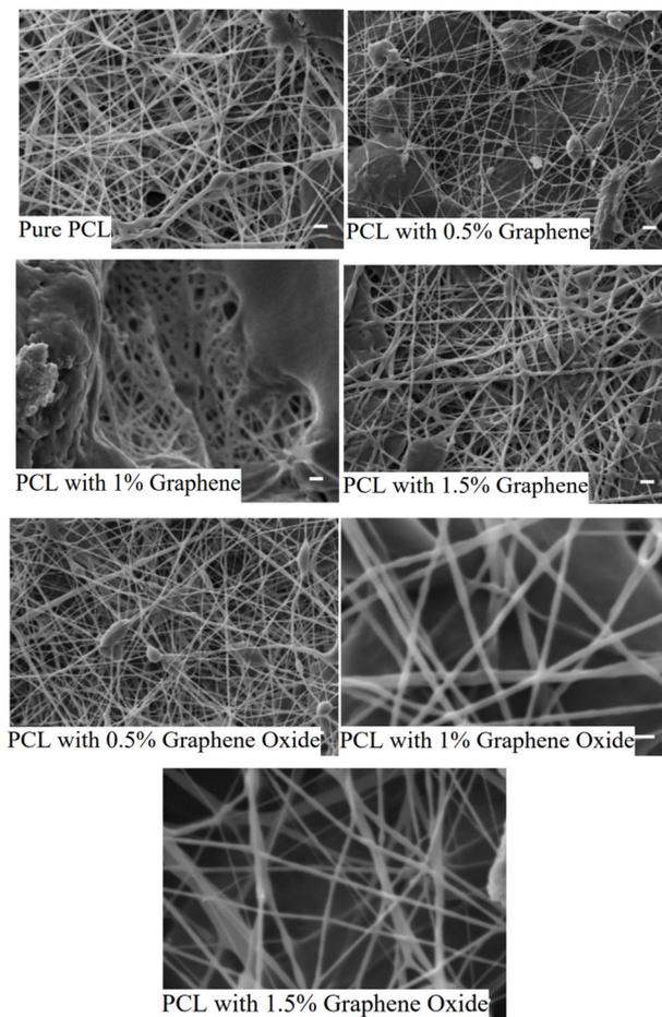
Figure 3: SEM images of electrospun PCL nanocomposite nanofibers.
