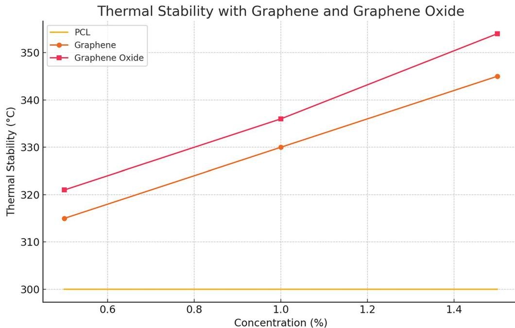
Figure 7: Thermal Stability with Graphene and (GO).
