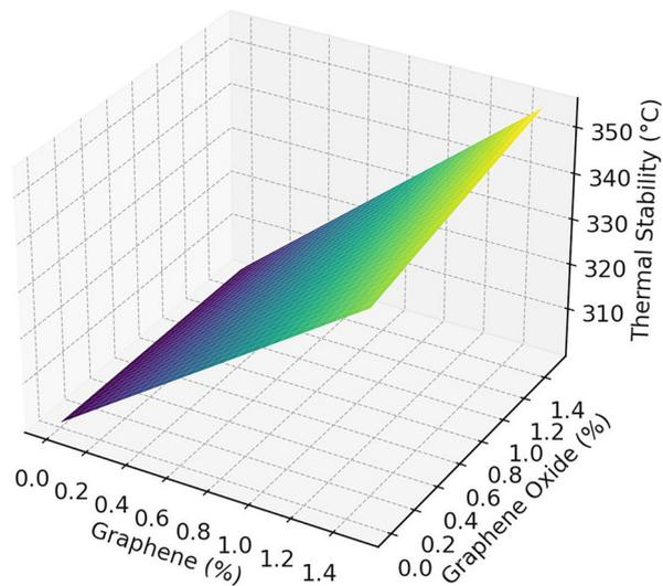
Figure 10: Response surface for thermal stability.
