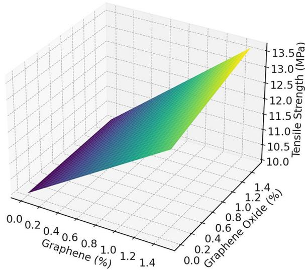
Figure 9: Response surface for tensile strength.
