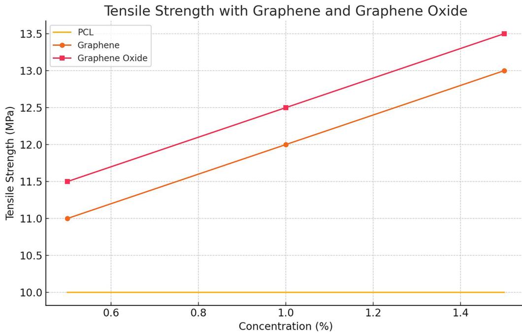
Figure 6: Tensile Strength with Graphene and (GO).
