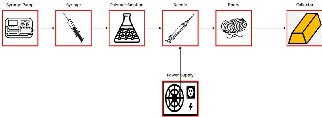
Figure 2: Schematic diagram of the electrospinning setup.
