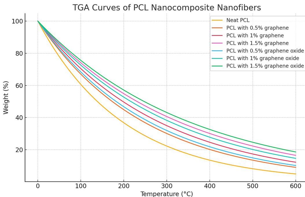
Figure 5: TGA curves of PCL nanocomposite nanofibers.
