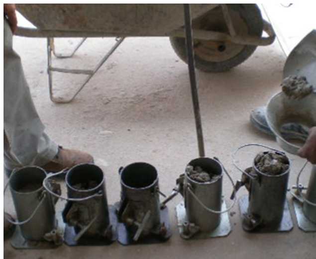
Figure 3: Molding of concrete specimens.
