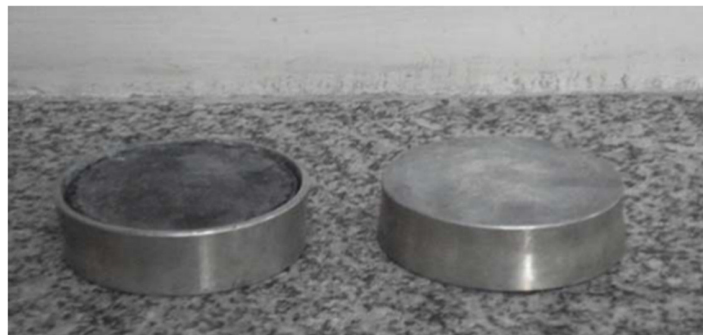
Figure 5: Neoprene disc – Replaces capping with sulphur.
