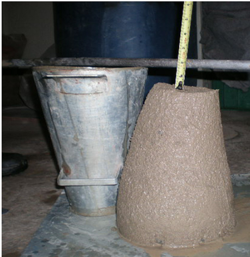
Figure 4: Determination of consistency by slumping the cone trunk.
