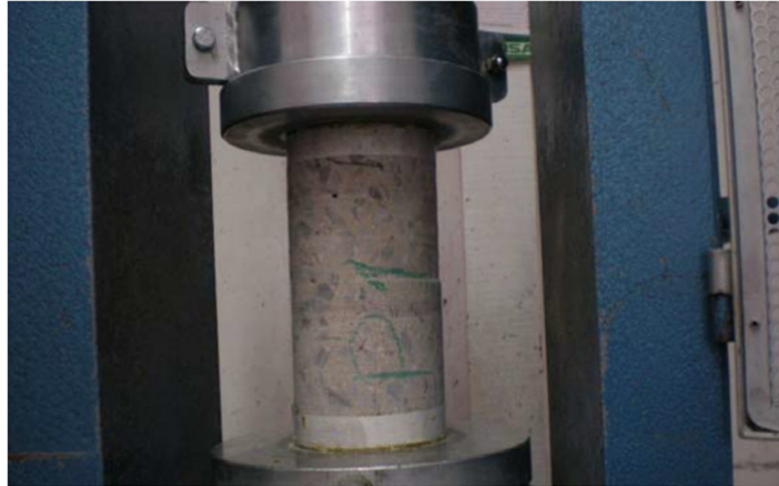
Figure 6: Regularization of the face with a neoprene disc.
