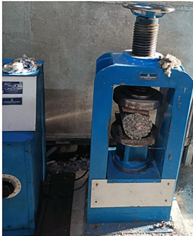
**Figure 2:** Splitting tensile strength test setup.
