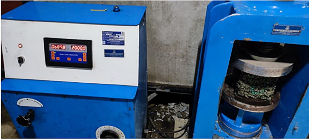
**Figure 1:** Compressive strength test setup.
