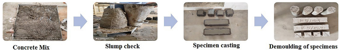
Figure 2: Manufacturing process of concrete specimen.
