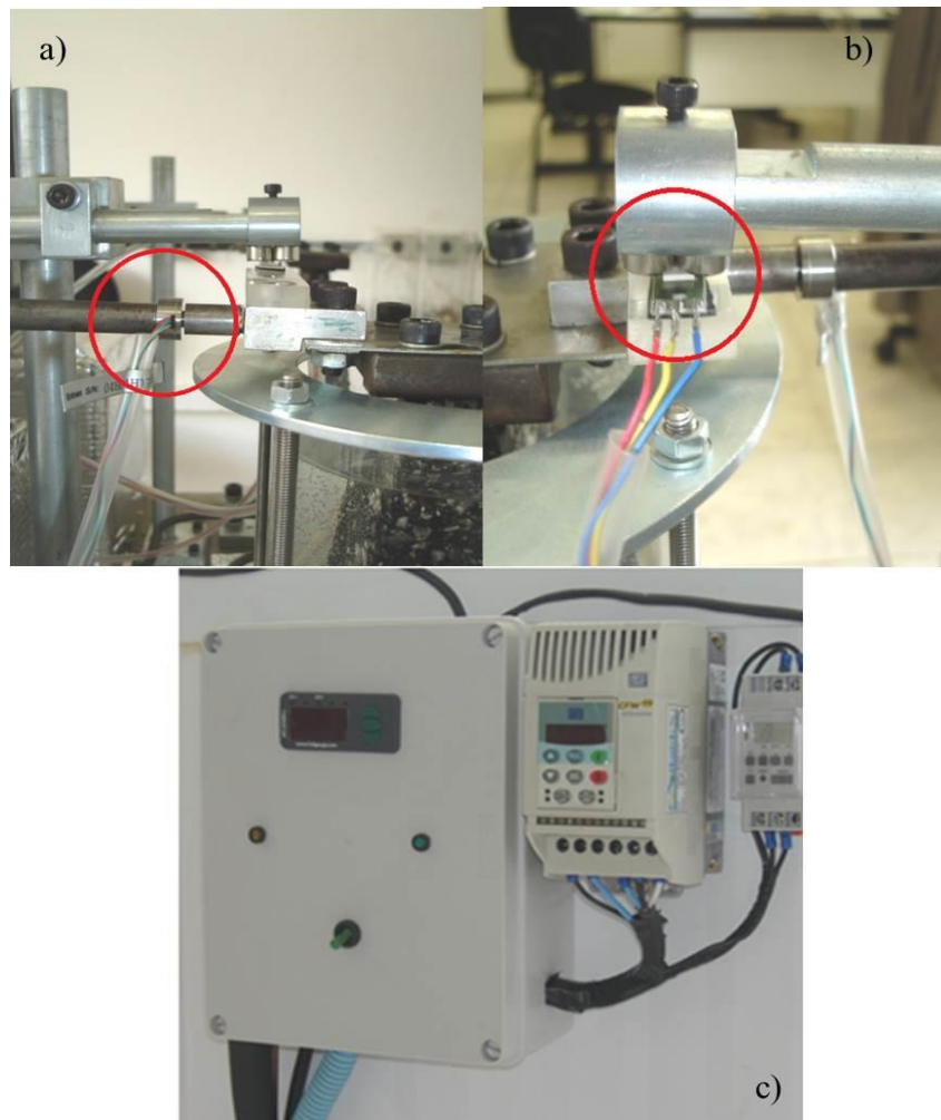
Figure 4: Detailed view of the: (a) loading cell, (b) Hall Effect sensor, (c) digital automatic controller (left) and frequency inverter (right).
