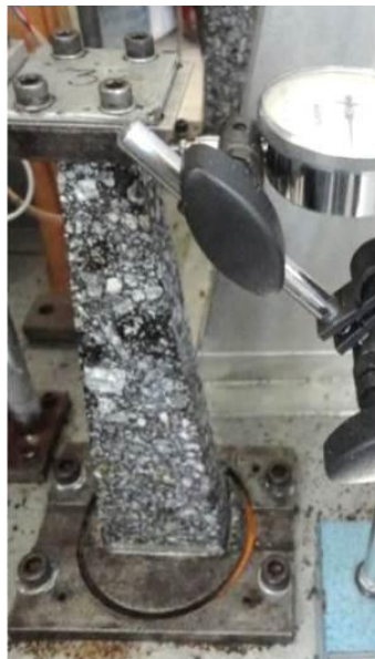
Figure 12: Adjustment of the displacement amplitudes using an analogical extensometer.
