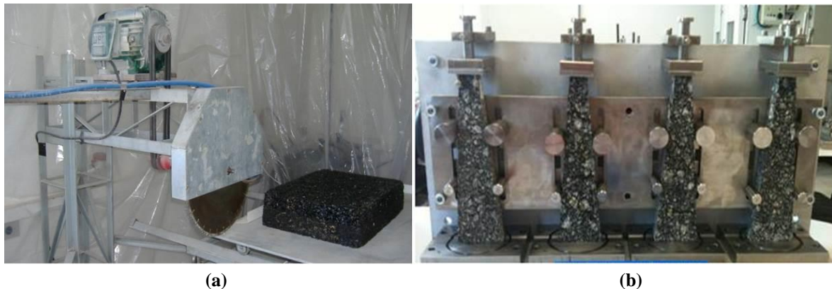
Figure 11: Overview of the (a) asphalt mix slab sawing procedure and (b) specimens selected for the tests.
