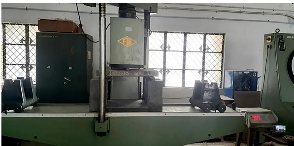
**Figure 11:** Load set up for static load test on slabs.
