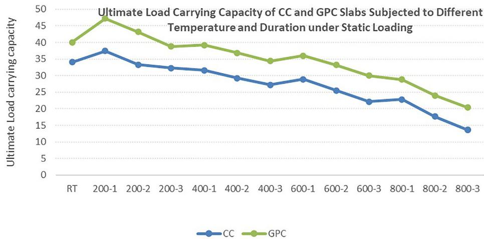
**Figure 15:** Overall comparison of Ultimate load carrying capacity of Cement and Geopolymer slabs at various temperatures and various durations.
