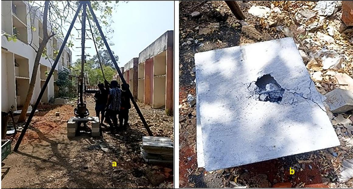
**Figure 16:** a) Impact load test set up. b) Punching failure of slabs by impact load test.
