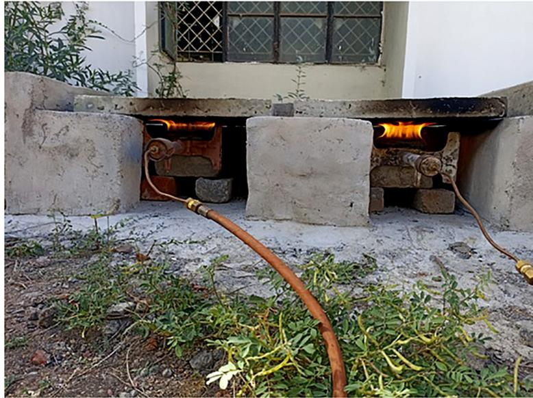
**Figure 9:** Exposure of fire on concrete slab.
