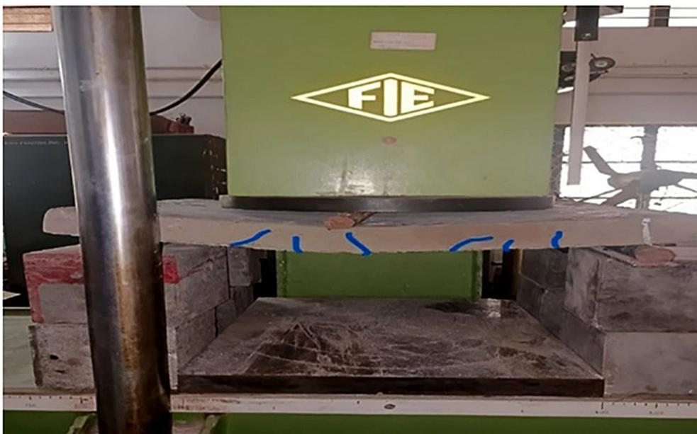
Figure 12: Failure mode of fire damaged slab.
