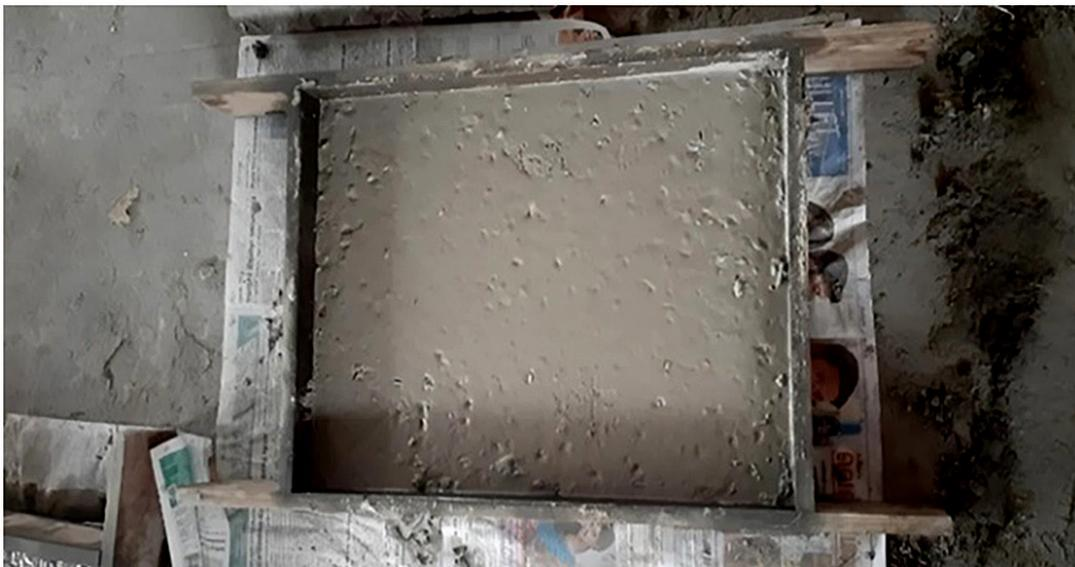
**Figure 4:** Casting of specimens.
