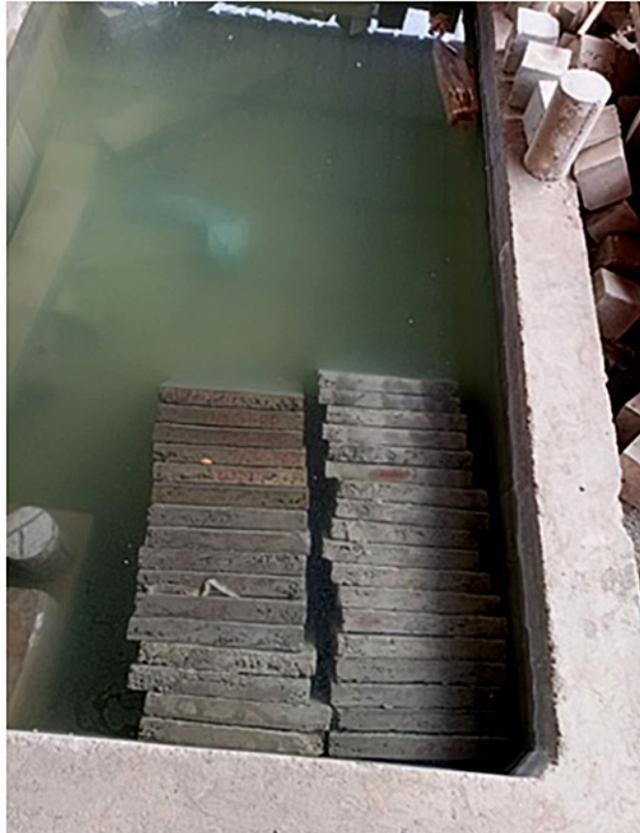
**Figure 5:** Water curing of cement concrete slabs.
