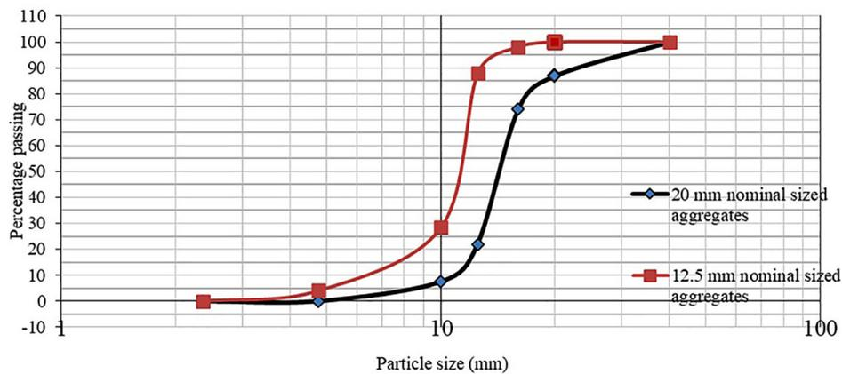
**Figure 2:** Gradation curve of coarse aggregate.
