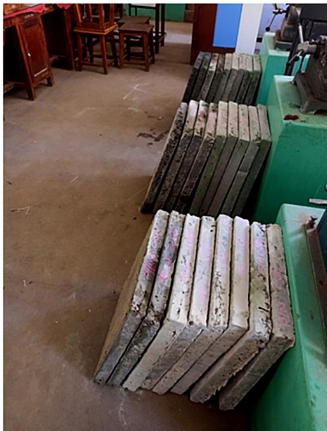
**Figure 6:** Ambient curing of geopolymer concrete slabs.
