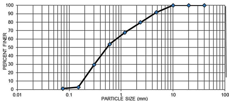
**Figure 1:** Gradation curve of fine aggregate.
