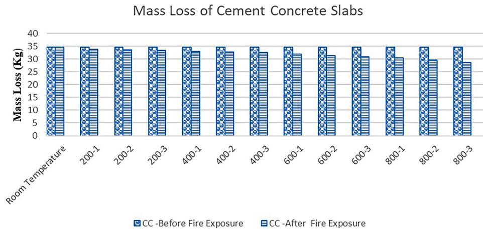
**Figure 13:** Mass loss of cement concrete slabs subjected to different temperature and duration.
