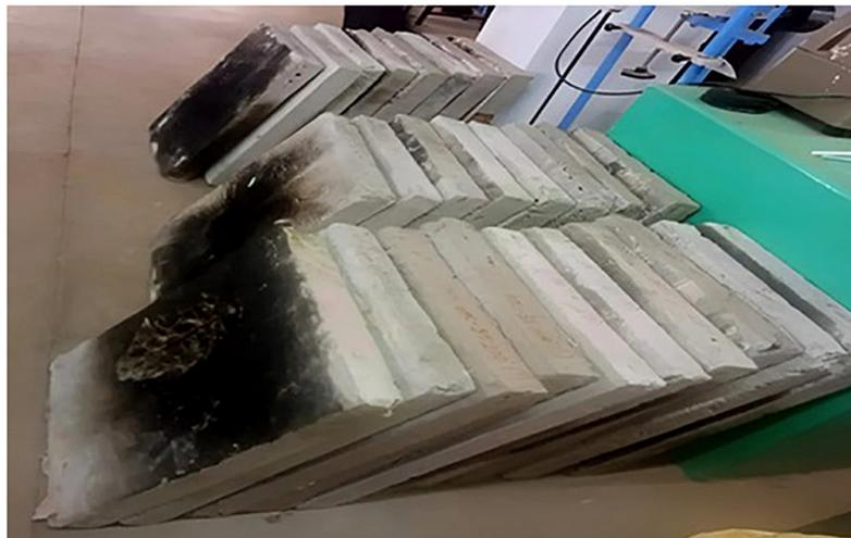
**Figure 10:** Fire damaged slabs.
