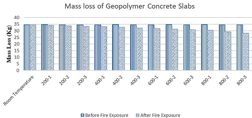
**Figure 14:** Mass loss of geopolymer concrete slabs subjected to different temperature and duration.
