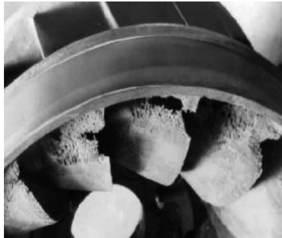
Figure 1: The blade cavitation phenomenon.
