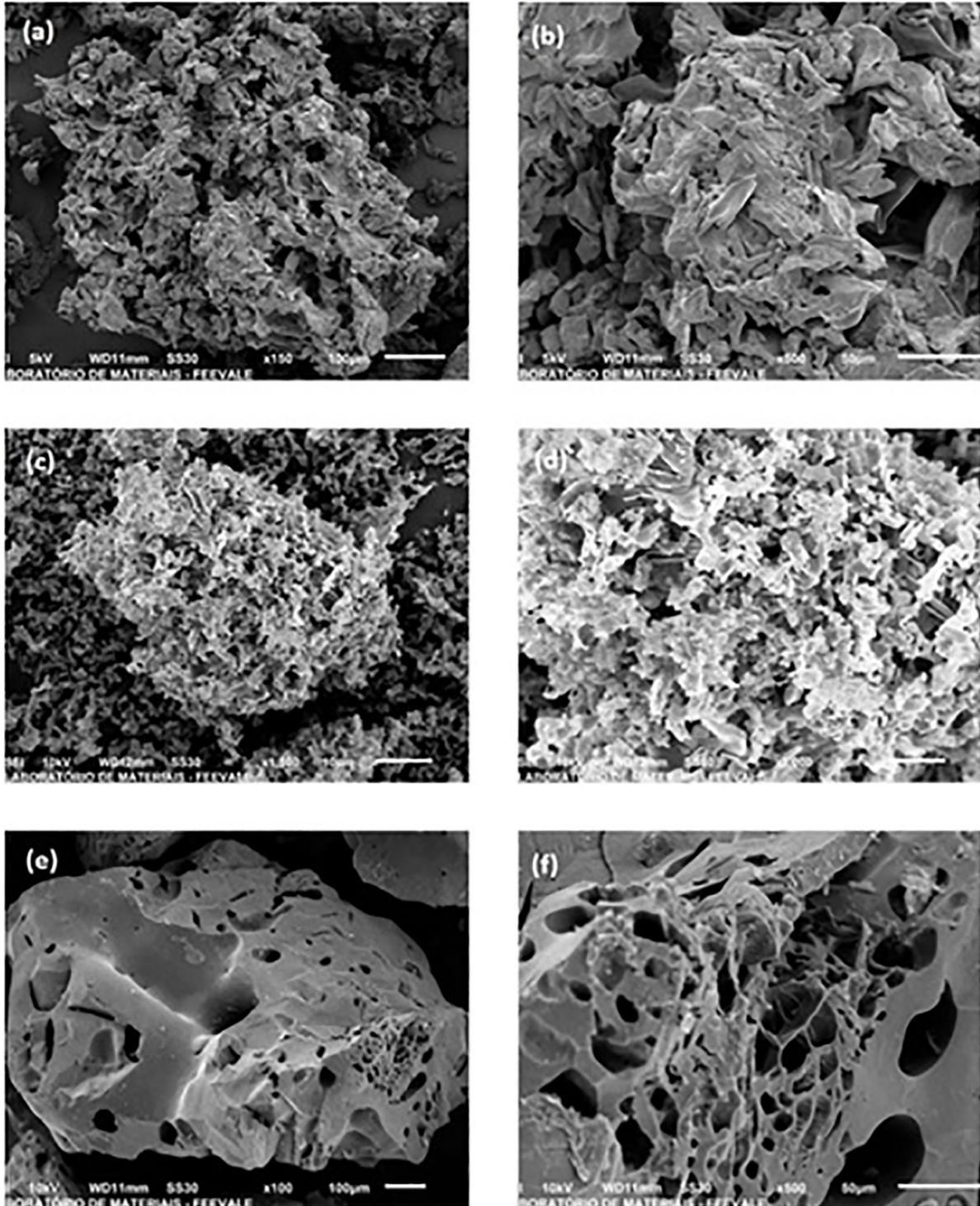
**Figure 2:** Micrographs of bioadsorbents developed from fresh orange peel, with magnifications (a) 150× and (b) 500×, thermally activated, with magnifications (c) 1500× and (d) 3000×, and chemically activated, with magnifications of (e) 100× and (f) 500×.
