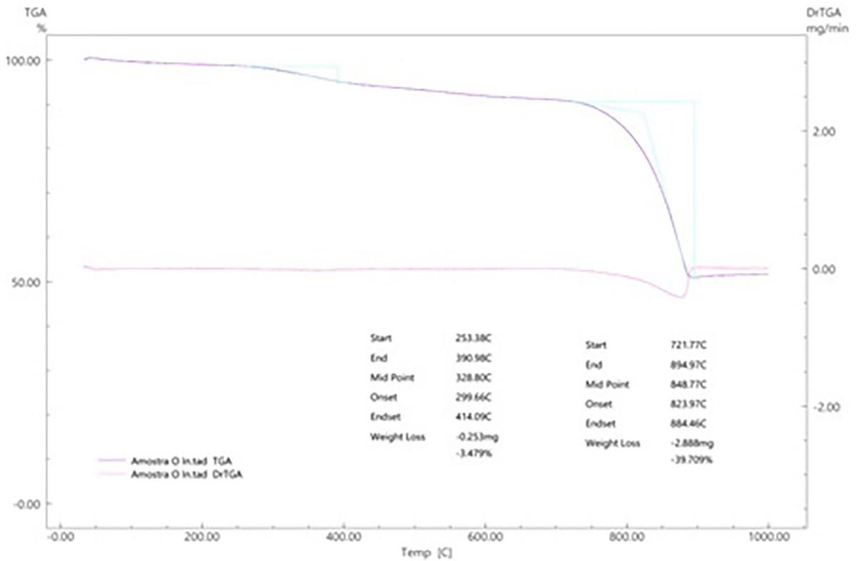
**Figure 6:** TGA/DTG curves of bioadsorbents developed from eggshell (a) in natura, (b) thermally activated and (c) chemically.
