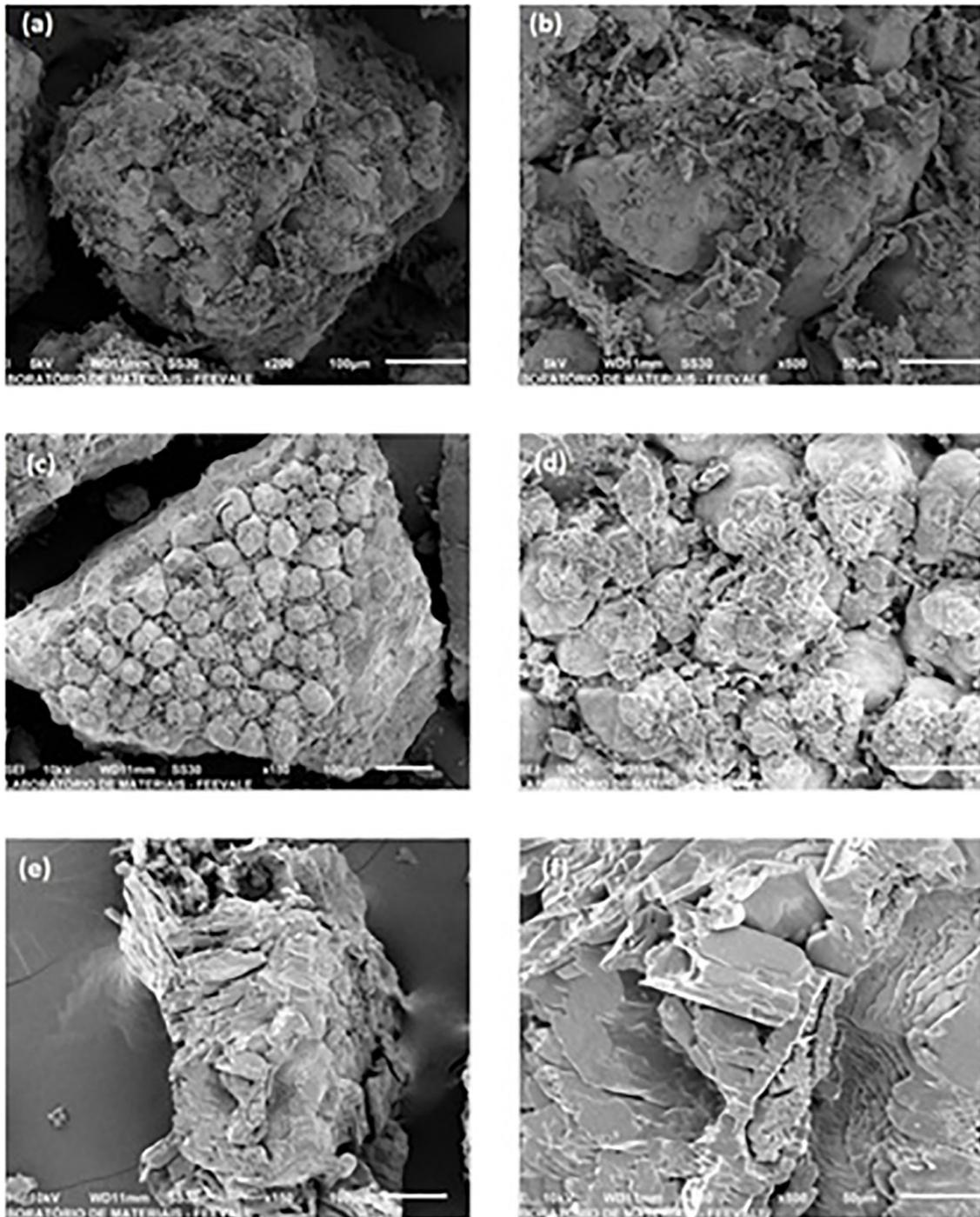
**Figure 3:** Micrographs of bioadsorbents developed from fresh eggshell, with magnifications (a) 200× and (b) 500×, thermally activated, with magnifications (c) 150× and (d) 500×, and chemically activated, with magnifications of (e) 150× and (f) 500×.
