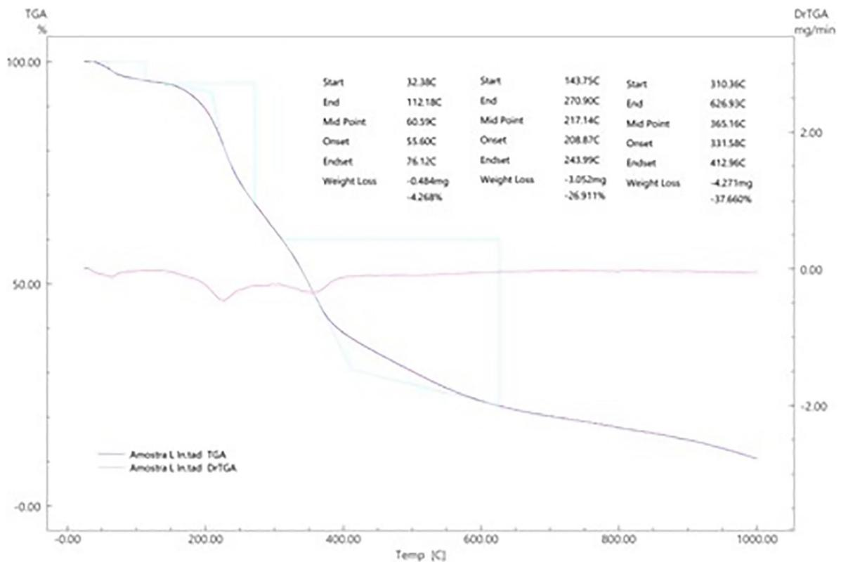
Figure 4: TGA/DTG curves of bioadsorbents developed from passion fruit peel (a) in natura, (b) thermally activated and (c) chemically.
