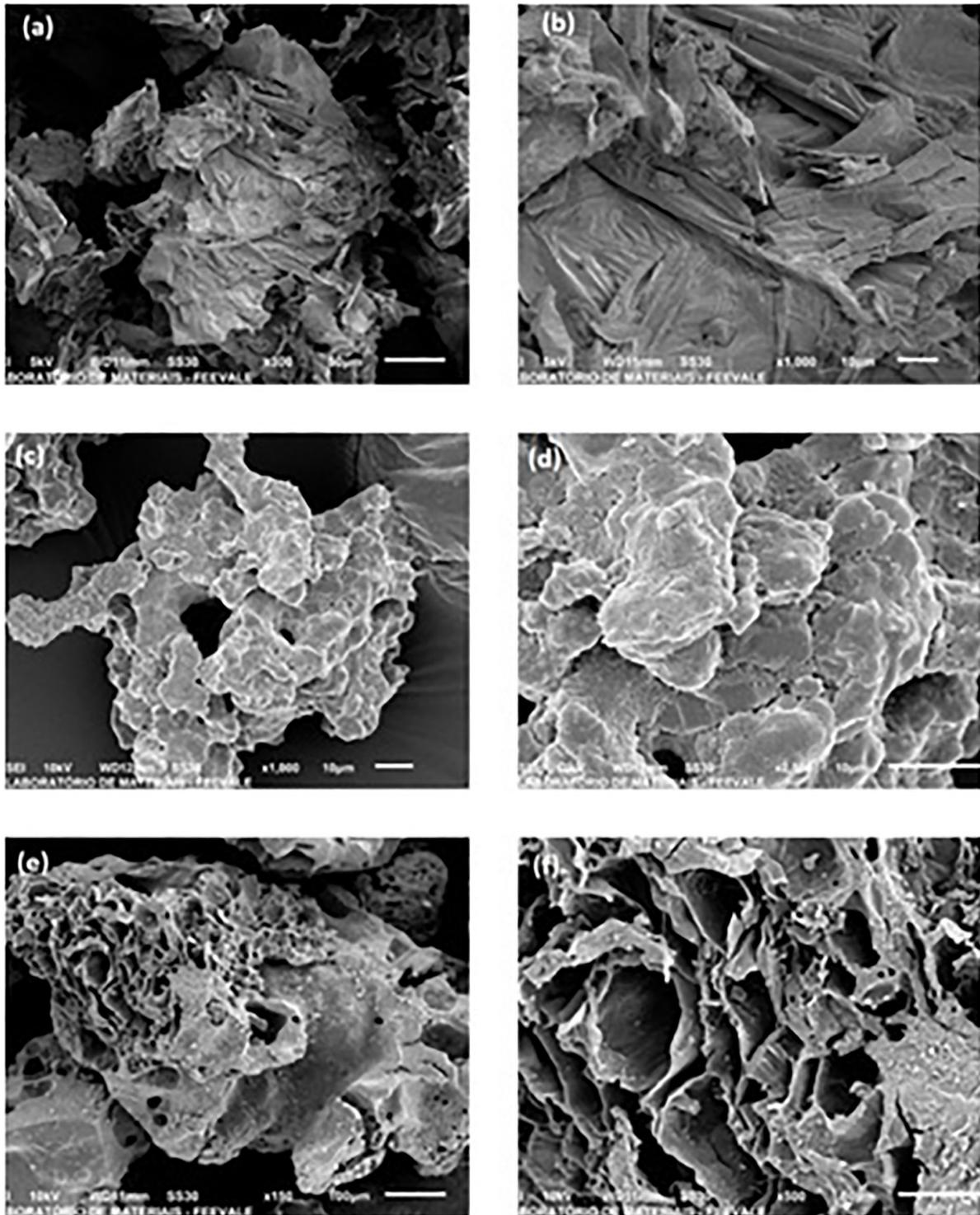
**Figure 1:** Micrographs of bioadsorbents developed from fresh passion fruit peel, with magnifications (a) 300× and (b) 1000×, thermally activated, with magnifications (c) 1000× and (d) 2500×, and chemically activated, with magnifications of (e) 150× and (f) 500×.
