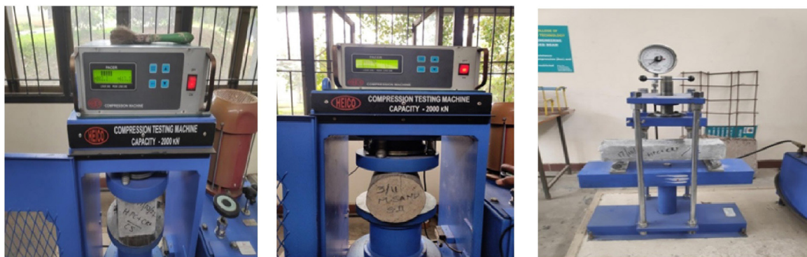
Figure 6: Mechanical property testing of HPCs specimens.
