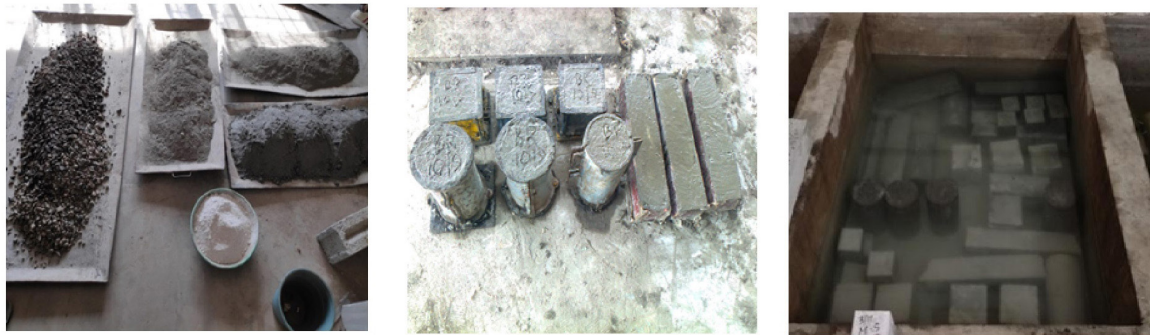
Figure 4: Casting and curing process of specimens.
