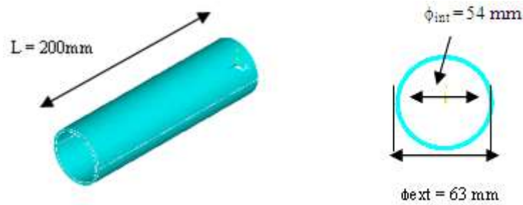
Figure 1: Geometry of tube piece specimen type, used for impact tests (falling weight).
