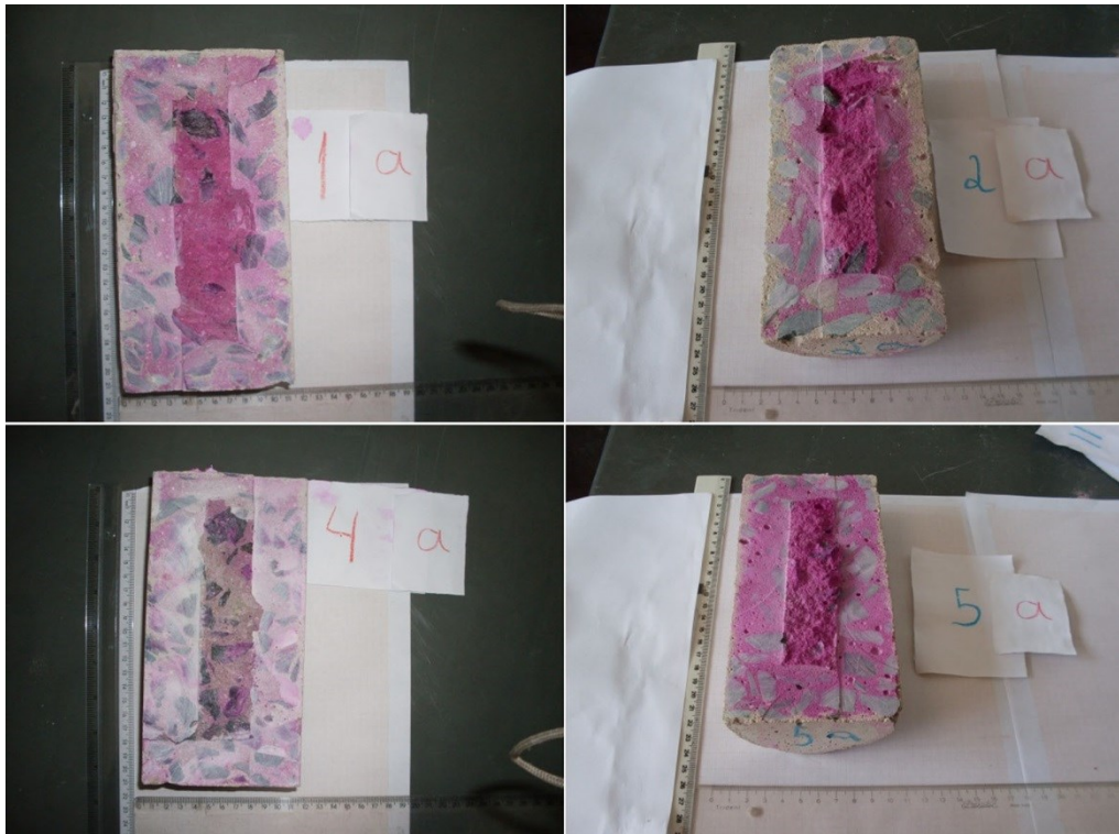
Figure 6: Carbonation depth of traces 1 (CPIII cement without MK), 2 (CPIII cement with MK), 4 (CPV cement without MK), and 5 (CPV cement with MK).
