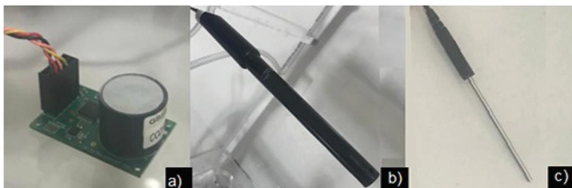
Figure 7: Sensors: a) CO<sub>2</sub> concentration; b) Humidity; c) Temperature.
