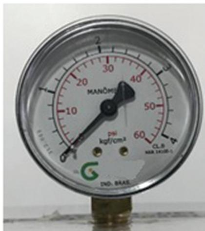
**Figure 8:** Pressure gauge to control the pressure inside the chamber.
