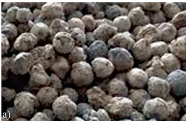
Figure 1: a) Fly ash aggregate b) microstructure of fly ash aggregate.
