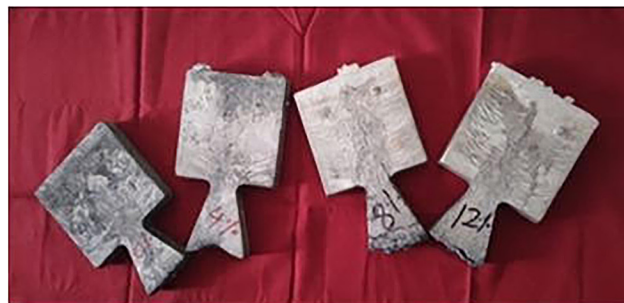
Figure 5: Fabricated ZK60/ZrB 2 composites.
