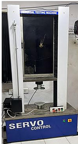
Figure 7: Universal testing machine for composite testing.
