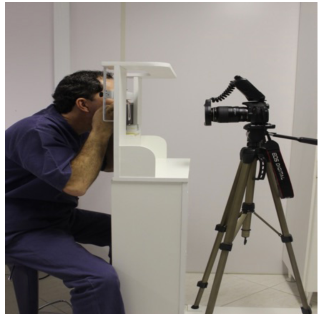
Figure 2. The position of the camera was also standardized using the device, since it has space for attaching the tripod, to establish the height and focal length of the camera.
