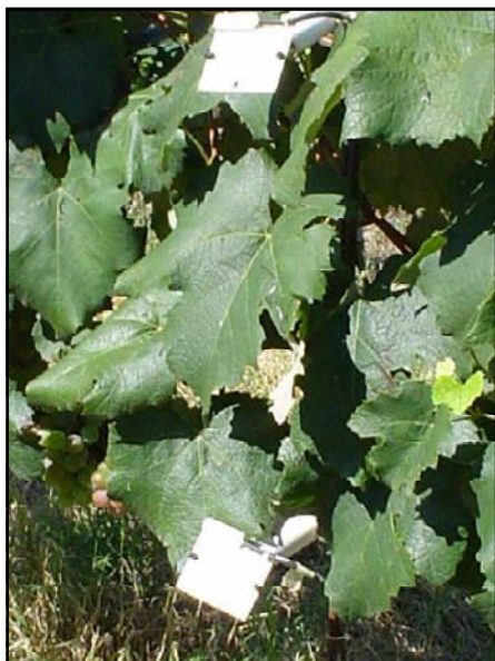
Figure 5 - Flat plate leaf wetness sensors installed in vineyard in Jundiá, SP, Brazil. (Photo: Jorge Lulu - 2005).
