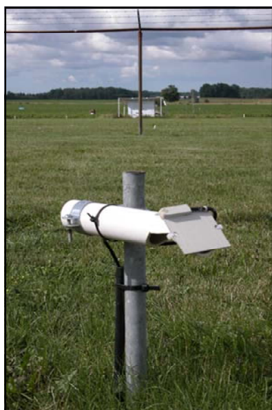
Figure 1 - Flat-plate leaf wetness sensor tipped 45 degrees from horizontal and exposed at 30 cm above turf grass.
