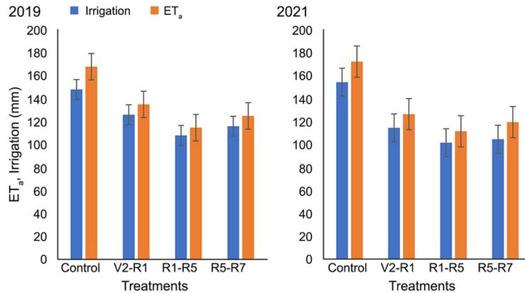
**Figure 3** – Irrigation depth, actual evapotranspiration ( $ET_a$ ) in different experimental treatments in two years. V2-R1 = water deficit applied from the second-node stage until the beginning of flowering; R1-R5 = water deficit applied from the beginning of flowering until the beginning of grain filling; R5-R7 = water deficit applied from the beginning of grain filling until the beginning of physiological maturation. Control = without water deficit.
