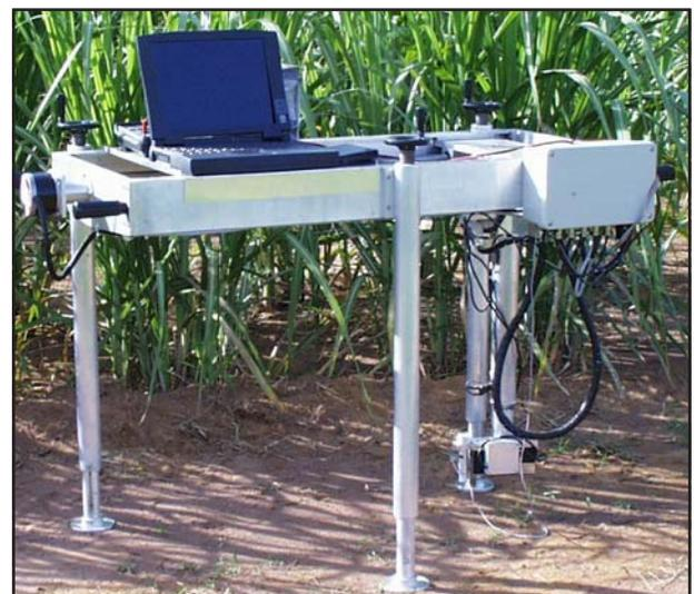
Figure 2 - Photograph illustrating a prototype of the intelligent instrument that captures and facilitates decisions regarding the evaluation of the resistance of soil to root penetration.
