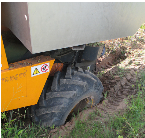
Figure 5 – Loss of trafficability in Plot 2 in Brazil due to soil moisture conditions.
