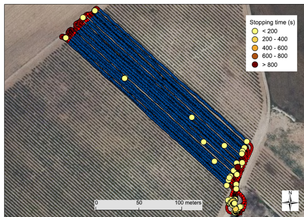
Figure 3 – Example of machine trajectories in plot number 16 (R41). Red lines refer to headland, blue lines to crop rows, and circles to machine stops with color referring to stop duration in seconds.
