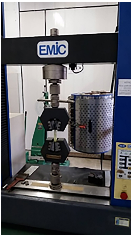
Figure 3 – Universal machine UMMT for testing mechanical properties of biological material with a stem being tested.
