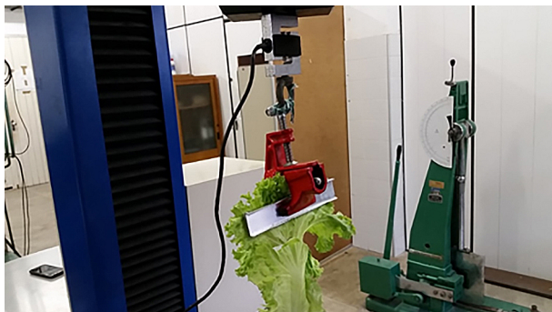
Figure 5 – Experimental setup for testing the lettuce leaves with the adapted lathe pulling a specimen. Note the rupture of the leaf far from the pressing elements, which proves the adequacy of the adaptation.
