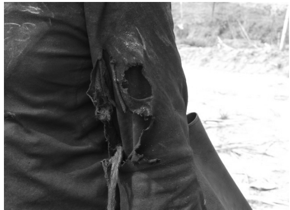
Figure 4 - Ripped protective sleeves
