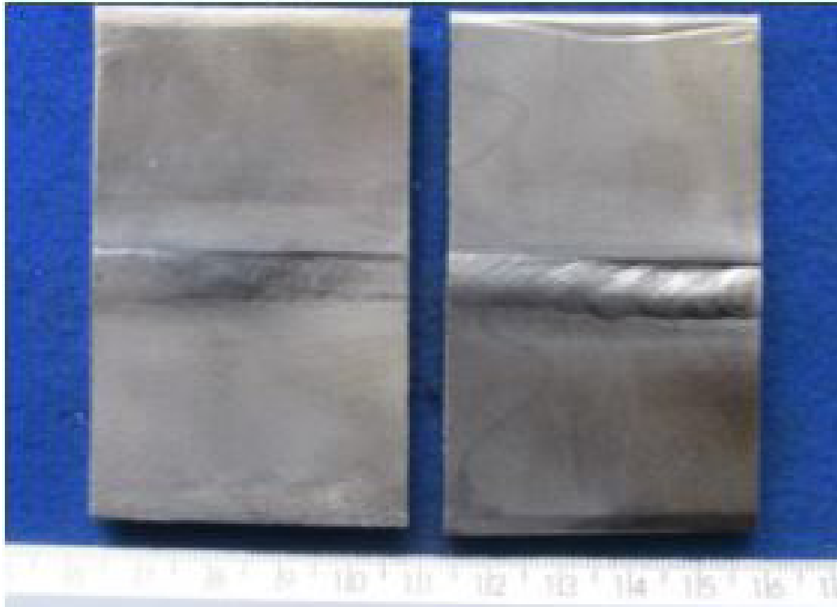
Figure 5. Visual testing of the welded joints after GTAW process.
