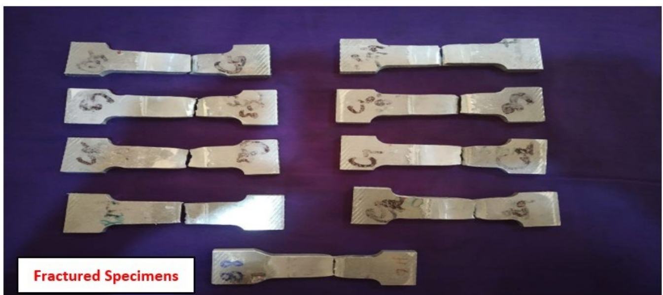
Figure 4. Fractured tensile samples of AA6082 and Cr 3 C 2
