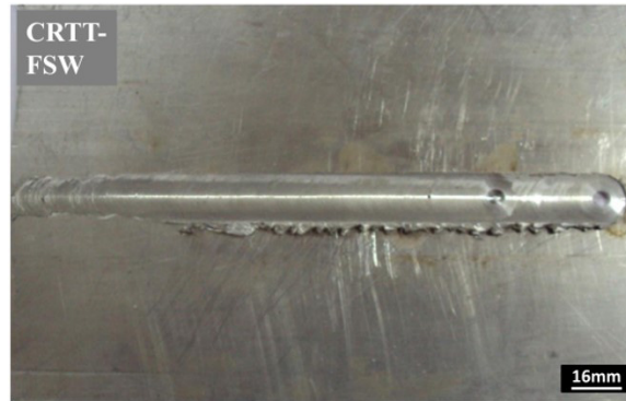
Figure 15. Weld joint obtained from counter-rotating twin tool [125].
