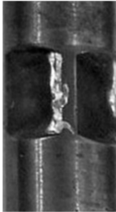
Figure 25. Cylindrical 4 Flat (square) pin profile [168].
