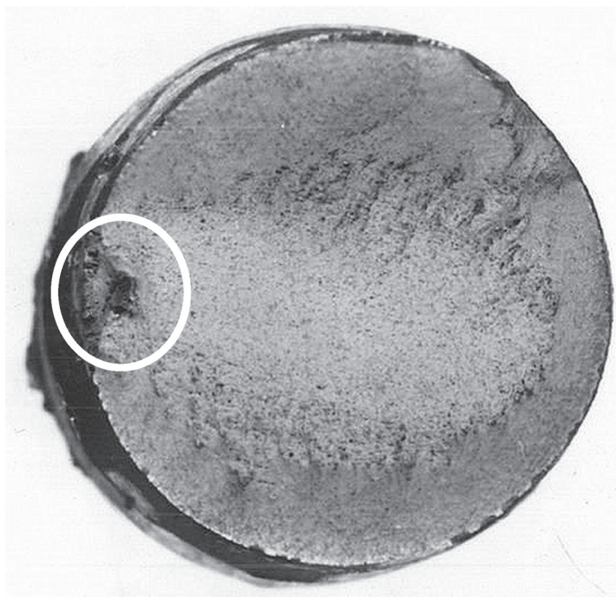
Figure 3. Fracture of reinforcement with a burnt spot
