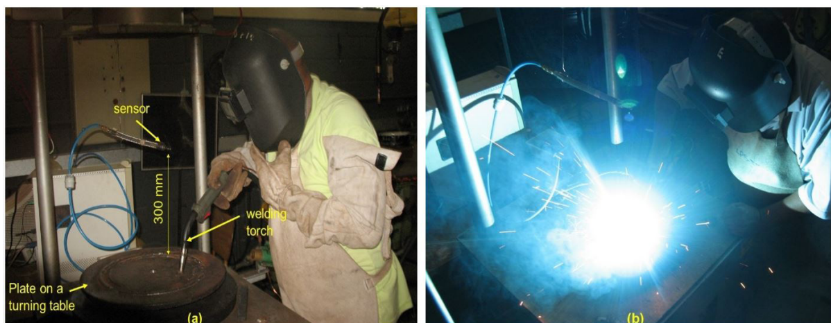
Figure 3. Sensor placed \approx 300 mm above the plate and over the arc: (a) without arcing; (b) with arcing.
