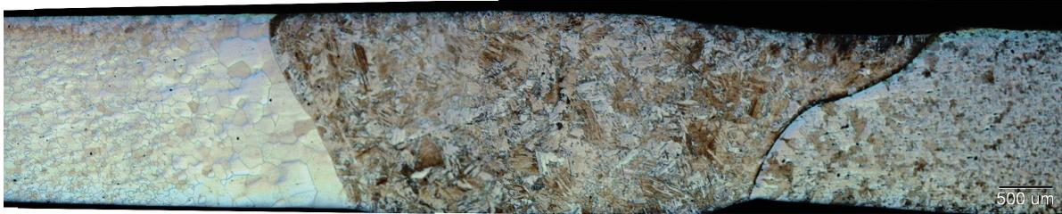
**Figure 9.** Weld pool obtained from metallography.
