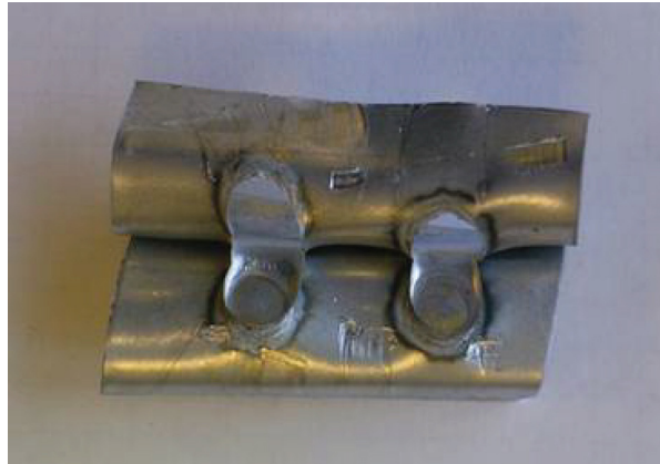
Figure 7. Fully automatic welding of mild steel plates, 0.7 mm / 0.7 mm.
