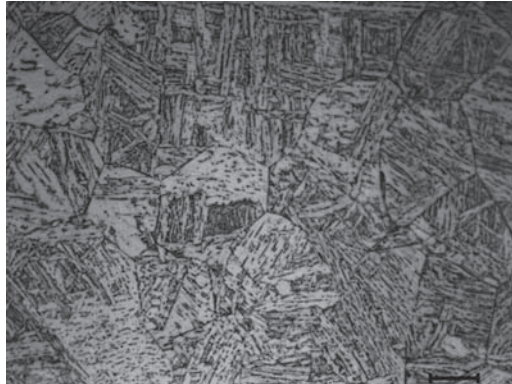
\Phi_{8.5} = 35 \text{ }^\circ\text{C/s} (20 µm): Dilatometer Lab B -Characterization Lab L
