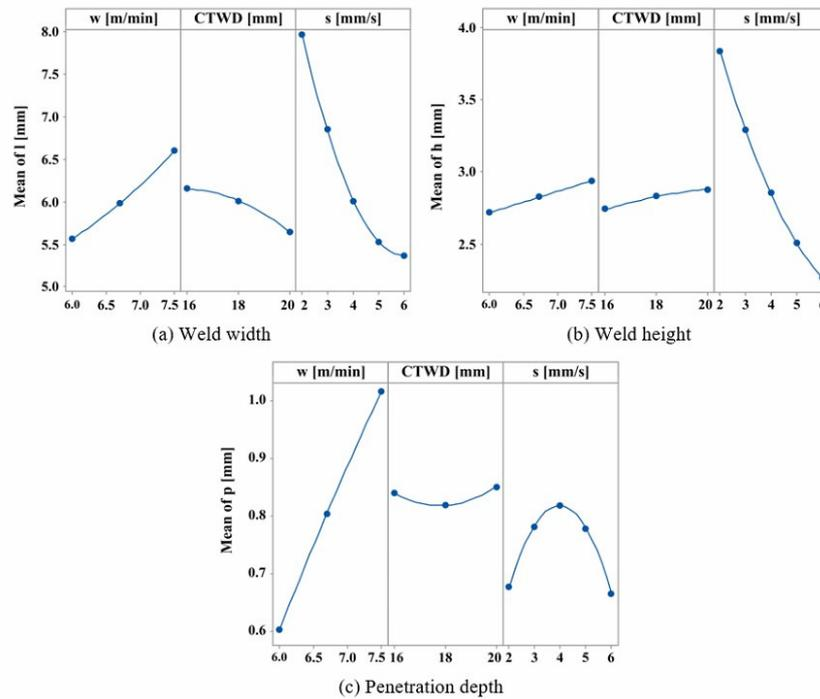
Figure 5. Effect of parameters in the bead geometry.
