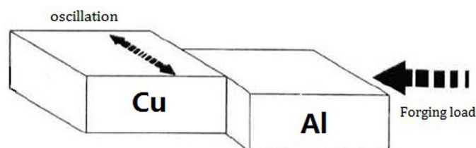
Figure 1. Schematic diagram of LFW process.
