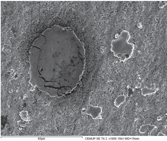
Fig 4 . Melted silver paste adherent to NiTi coupon
