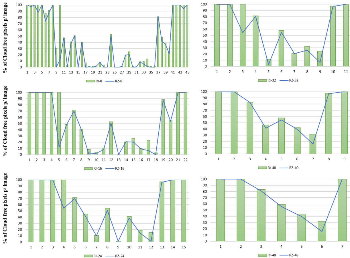
Figure 6 - Comparison between compositions with regular intervals (with and without the use of zenith sensor angle restriction) considering the percentage of valid pixels in the composition.
