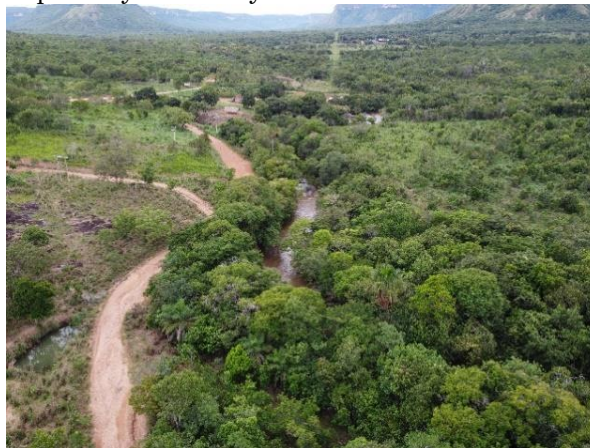
Figure 8 – High susceptibility caused by the confluence of roads and drainage network.
