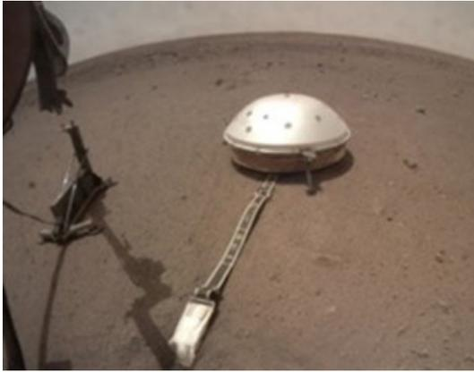
**Figure 3.** Image taken from the Instrument Context Camera (ICC) on sol 87 (local time 11:54:07 LMS) showing the location of SEIS and of the HP<sup>3</sup> support structure, 1.18 metre apart from each other (image credit: JPL/NASA).
