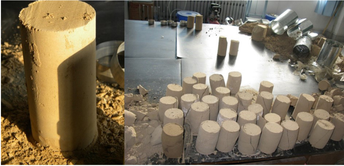
Figure 2. The preparation process of undisturbed soil and the soil samples after shear failure.
