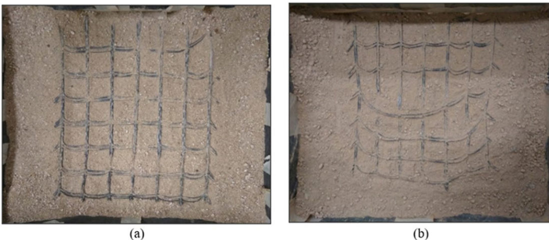
Figure 10. Exhumation of the geogrids used in the pull-out test ( \sigma = 50 kPa): (a) NS and (b) GRS-200-D.
