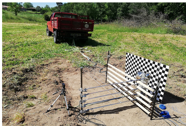
Figure 13. Test set-up used for the in-situ testing of the posts.
