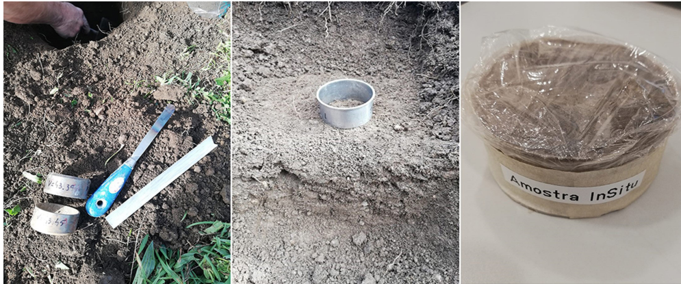
Figure 3. Extraction of undisturbed in-situ specimens.
