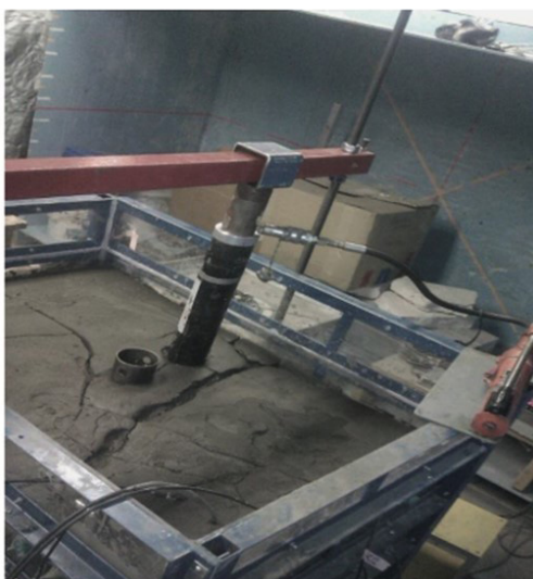
Figure 4. Drying box test (1m × 1m in plan) showing extraction of samples with thin-walled tubes (from Daliri et al., 2016).
