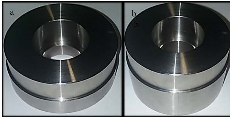
Figure 6. (a) Steel ring in steel rock centering ring and (b) steel ring in steel support ring.
