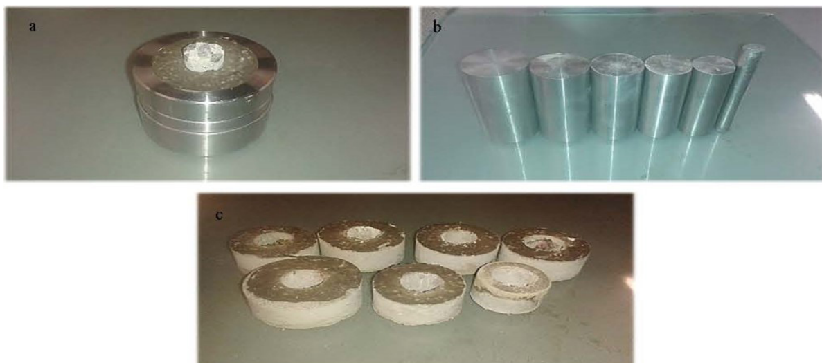
Figure 9. (a) Specimen on steel support ring ready for testing, (b) Steel rods for driving out the substrate and liner, and (c) Liner driven out of the steel ring after testing.
