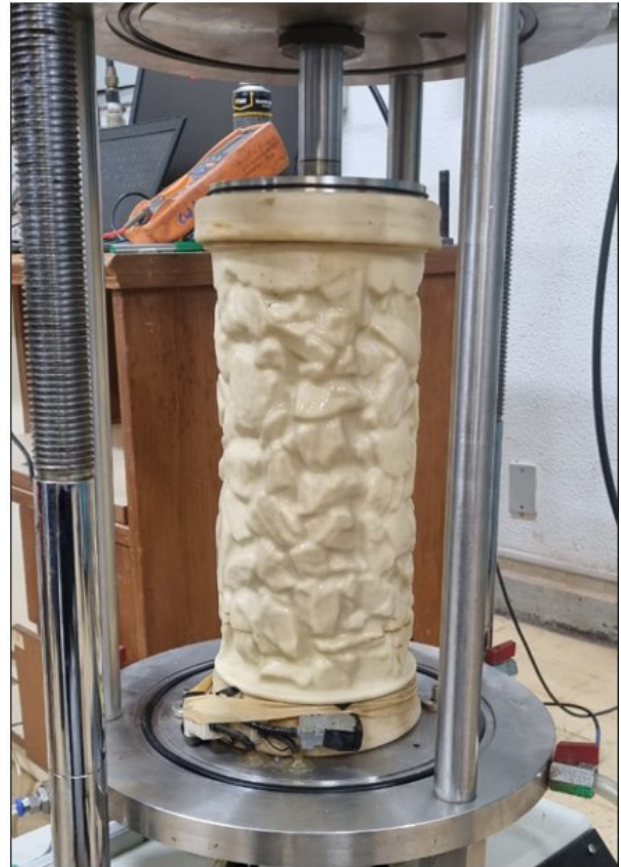
Figure 3. Specimen prepared for monotonic triaxial tests.
