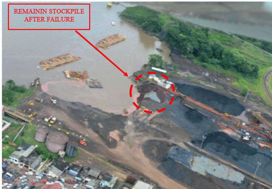
**Figure 4.** Post-failure scenario, highlight for the remaining stockpile (modified from Brasil, 2014).
