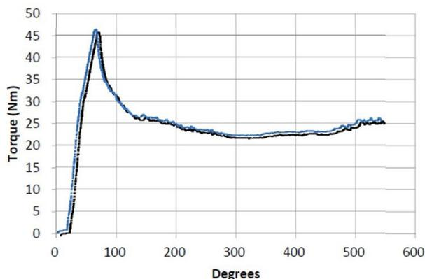
**Figure 9.** Typical vane test plot from the site (Pacheco et al., 2014).
