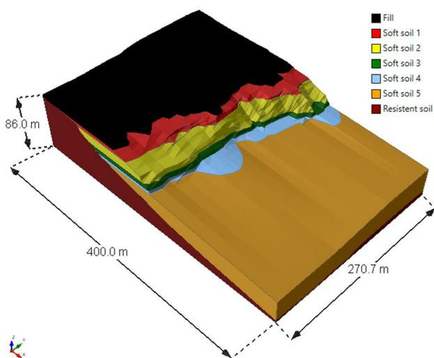
Figure 15. Three-dimensional slope model (adapted from Silva, 2021).
