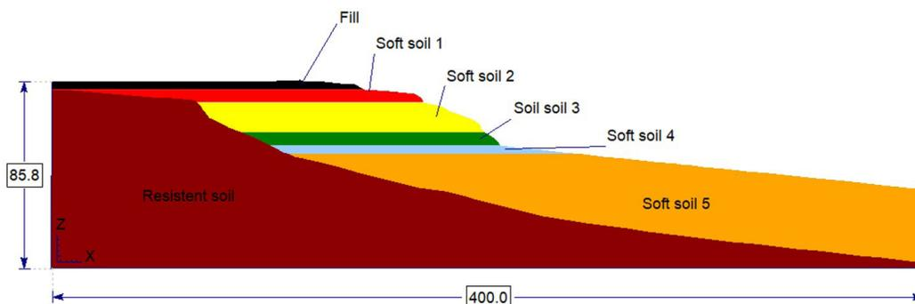
Figure 17. West cross section, drawn from the three-dimensional model.
