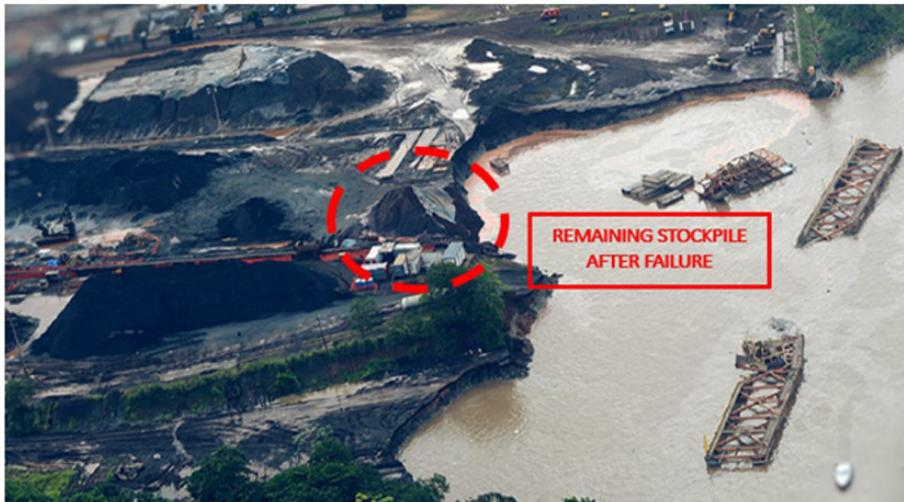
**Figure 6.** Post-failure scenario, both West and East sides. Highlight for the remaining ore Stack (adapted from Pacheco, 2017).
