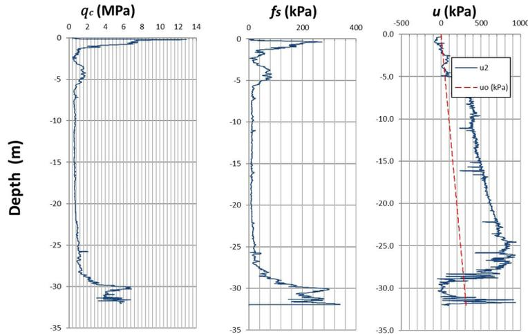
Figure 11. Basic CPTu data for one borehole -  $q_c$ ,  $f_s$  and  $u$ .
