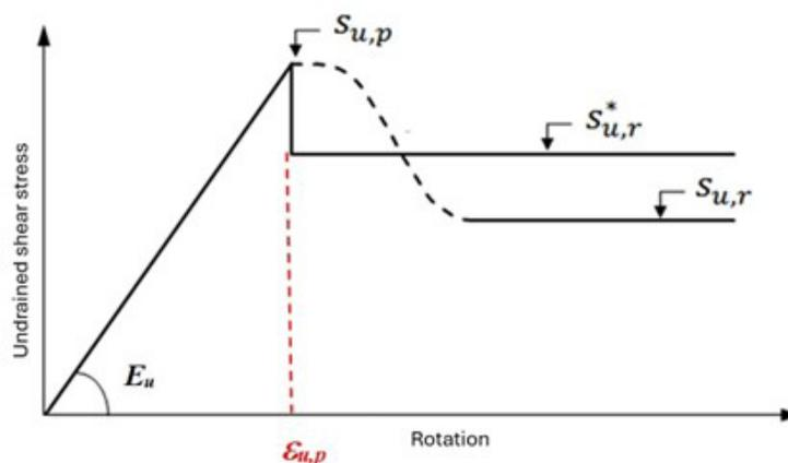
**Figure 1.** Equivalence between stress vs. rotation curve of the abrupt loss model and the real behavior in vane test (Pereira Pinto, 2017).
