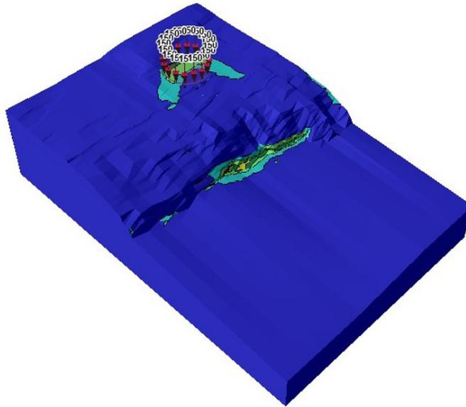
Figure 18. Contours of maximum shear strains at failure, for the analysis with stockpile loading and strain-softening (Silva, 2021).
