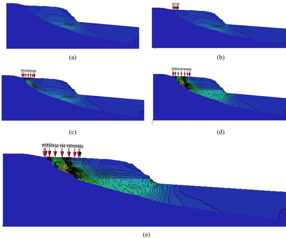
Figure 20. Maximum shear strains as loading increases: (a) initial condition, no load; (b) load with radius of 7.5 m; (c) load of radius of 17.5m; (d) load of radius of 25 m; (e) load with radius of 50 m (Silva, 2021).
