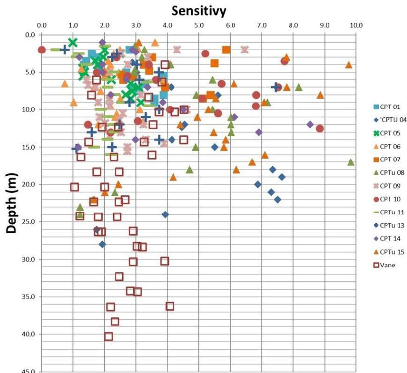
**Figure 10.** Soil sensitivity obtained by vane tests and correlation with CPTu tests (adapted from Pacheco et al., 2014).
