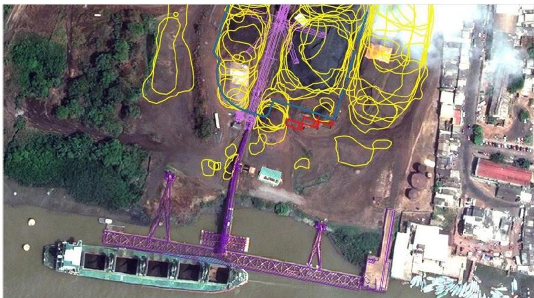
**Figure 3.** Overlapping of stacks between January and March 2013. The boxes in red indicate the boundary between the soft soil and the resistant soil, according to forensic studies (Pacheco, 2017).
