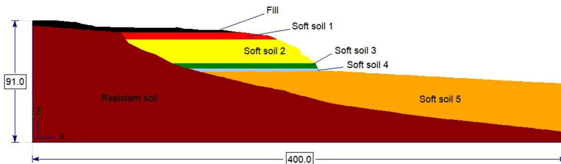
Figure 16. East cross section, drawn from the three-dimensional model.
