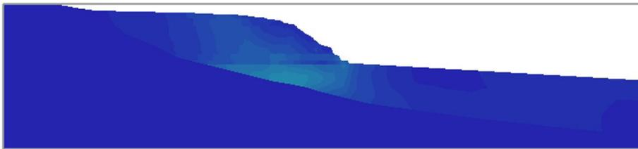
Figure 19. Maximum shear strains - no loading and no strain-softening,  $FS = 1.8$  (Silva, 2021).
