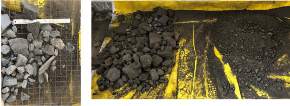
Figure 4. Sieving of through 30 mm sieve and amount retained and passed through 30 mm sieve.
