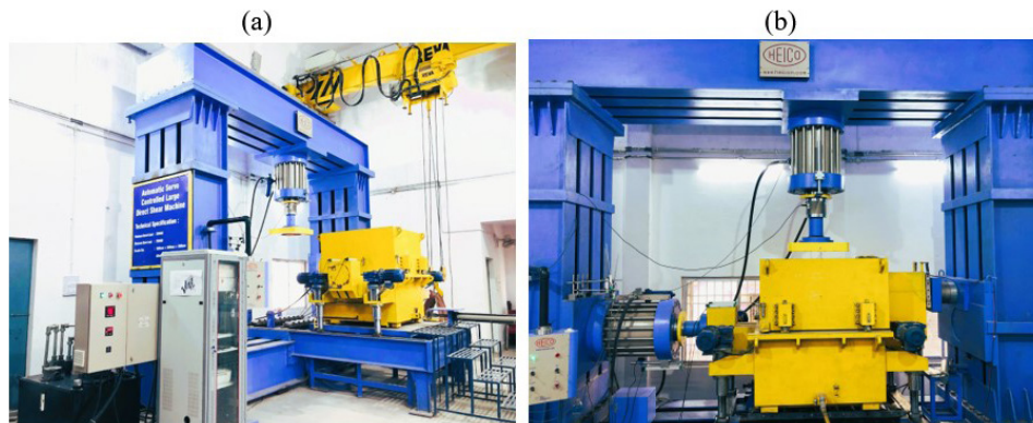
Figure 10. (a) shear box in position for loading of the sample; (b) shear box in position for application of normal and shear loads.
