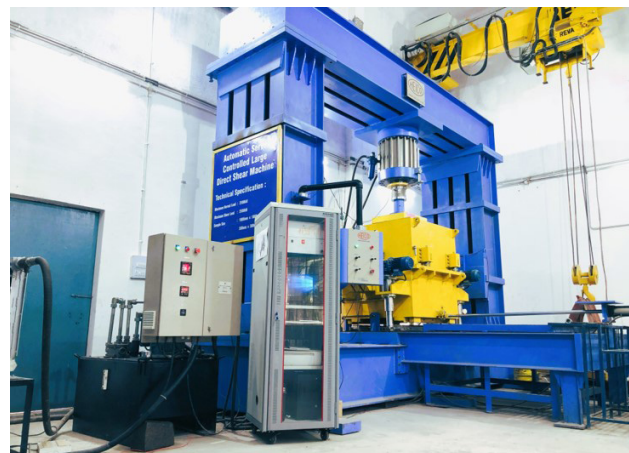
Figure 9. View of the large direct shear machine installed at CMPDI.
