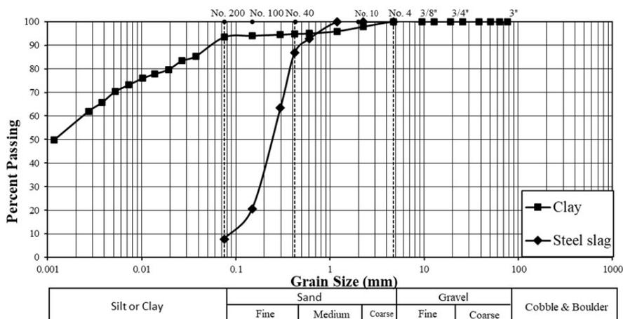
Figure 1. Grain size distributions of Tabriz soil and steel slag.
