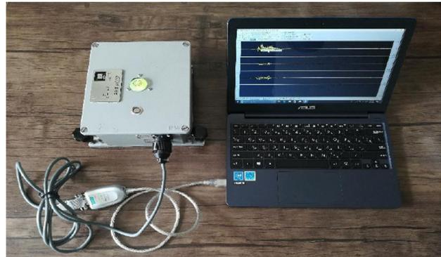
**Figure 6.** Setup illustration of GS11D sensor with an internal 12V rechargeable lead battery connected to a laptop.
