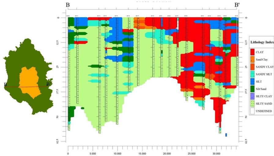
Figure 4. The lithology of the east-west cross-section between boreholes no. 20 to 185.
