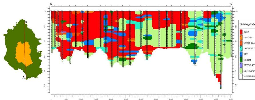
Figure 5. The lithology of the north-south cross-section between boreholes no. 400 to 062.
