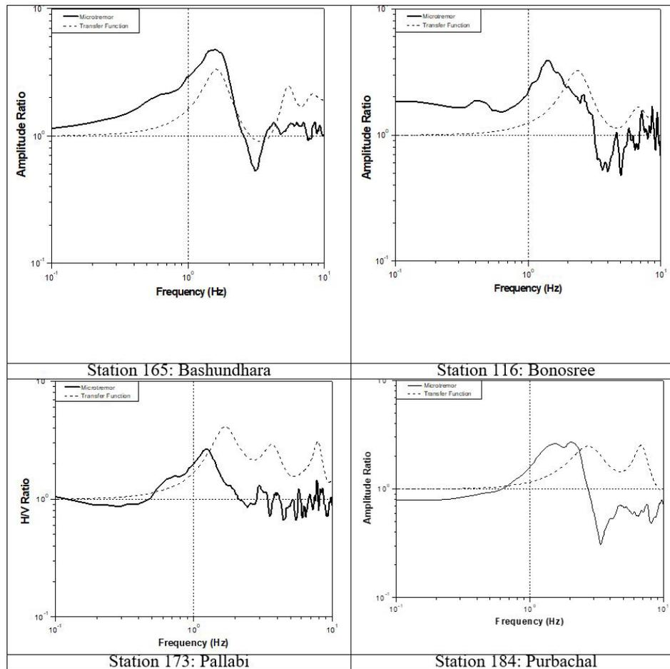
**Figure 12.** Comparison of  $H/V$  peak amplitude of microtremor and theoretical transfer function from numerical 1D response analysis for various locations in Dhaka city.
