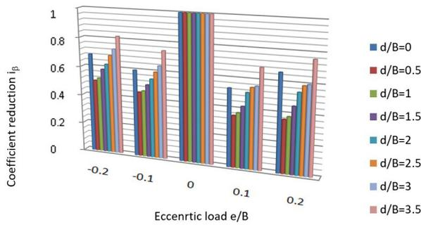
**Figure 11.** Variation of Reduction factor  $i_\beta$  as a function of the ratio of eccentricity  $e/B$ .
