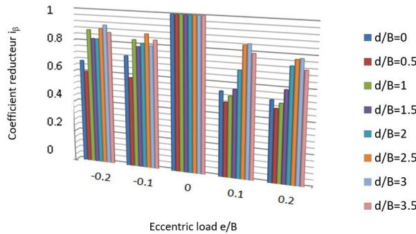
**Figure 13.** Variation of Reduction factor  $i_\beta$  as a function of the ratio of eccentricity  $e/B$ .
