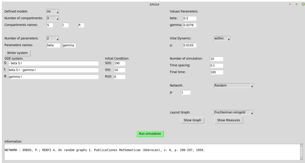
Figure 2: The EPIGUI interface. In this interface, the user is able to set up the number of compartments, parameters and write the correspondent equation. Additionally, the type of network and respective parameters are also disposable to be configured.
