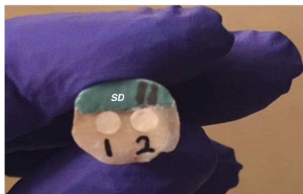
Figure 1. One tooth as a specimen with prepared and filled round cavities, one cavity received pretreatment with biomimetic analogs and the other did not receive. It also shows area of protected sound dentin (SD) with blue varnish to be taken as reference within each specimen.
